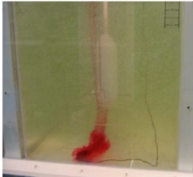
b) A Type 2 subsurface vortex forming from the back wall and entering Pump K. (6462)
