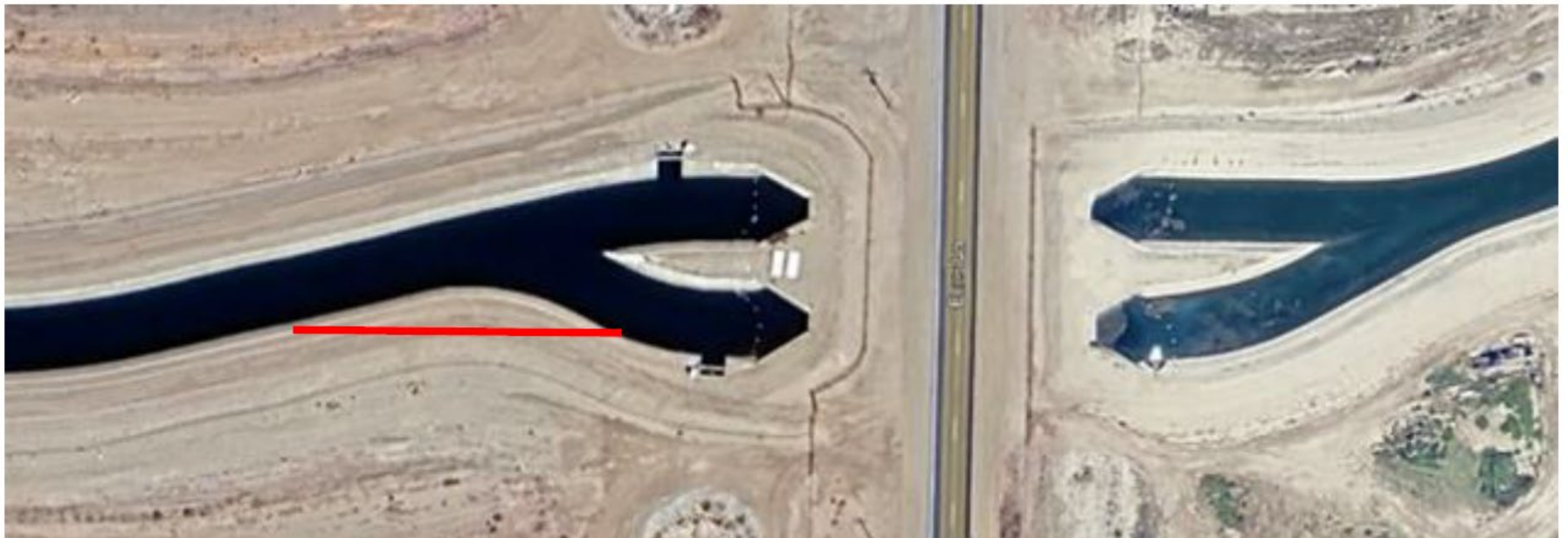
Figure 4. Enos siphon widening recommendation
