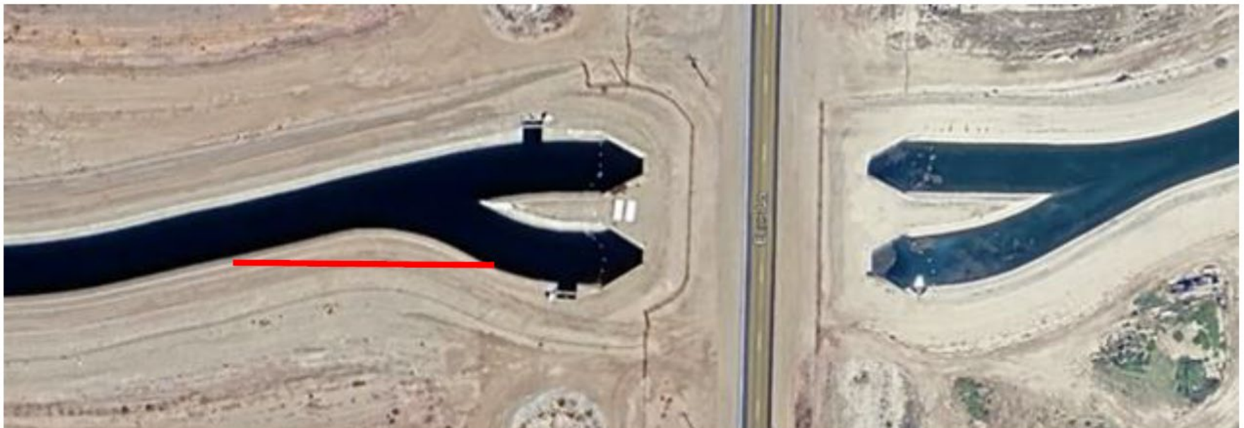
Figure 4. Enos siphon widening recommendation
