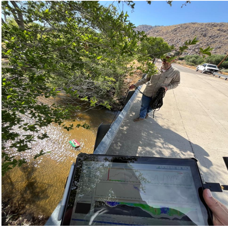
Figure 1 District Staff Performing Weekly Stream Gauging at South Fork
